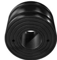
Standard glass-filled Teflon, O-ring energized piston seal with two bronze-filled bearing strips—installed on a ductile iron piston. (Code G)
